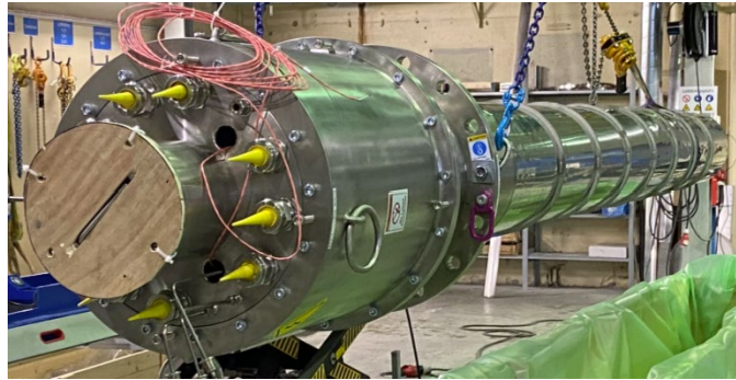
Figure 3: Pilot electric heater for the HYDRA IT06 project (Castel Romano, Italy)
